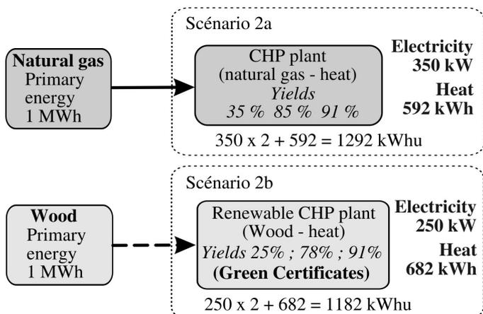
In scenario 2a, CHP cogeneration uses a gas turbine to generate electricity (electric yield 35%) and recovers 65% of the exhaust heat in an exchanger. The global electric yield could be 100% if the heat recovery did not have a weaker yield in the CHP heat exchangers (82%) than in separate gas boilers (90%). The global electric yield is
