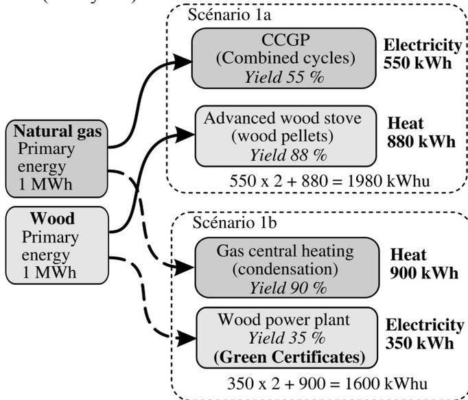
Scenario 1a is better than scenario 1b, since both use the same supply of energies but 1a produces more electricity, not because of environmental principles but because the gas turbines have a much more efficient technology than the steam power plants.
